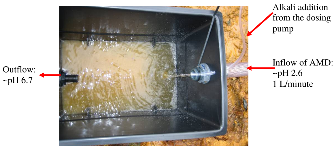
Figure 8.8. Alkali addition to the Ida mine drainage.
