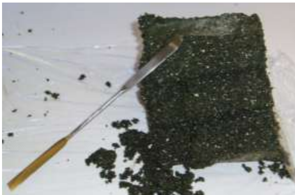
Figure 7.10. The core taken from the Bwlch 1 L/minute Algavi (c) DS bed.
